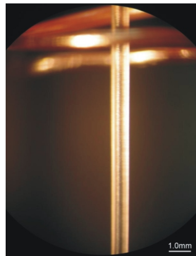
Figure 1: Single crystal fiber growth process.
