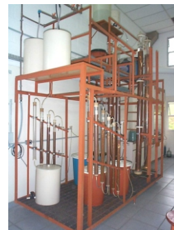
Figure 14. Assembly made to prepare high purity rare earth' oxides by ion exchange
