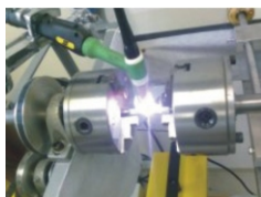
Figure 20. TIG welding on stainless steel filters
