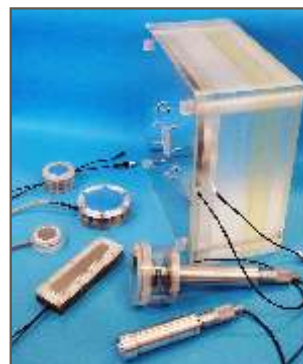
FIGURE 1 - Ionization chambers developed at IPEN.
