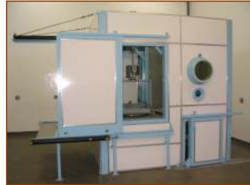
FIGURE 1 - Hot cell designed to handle sources.
