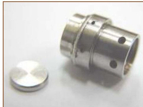
FIGURE 1 - Piece of a fuel injection nozzle drilled by the LMPC.
