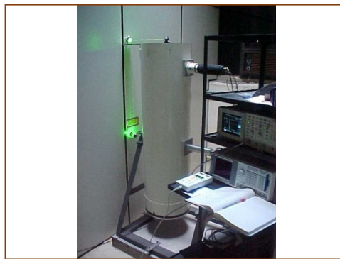
FIGURE 2 - Picture of the Lidar system in operation.
