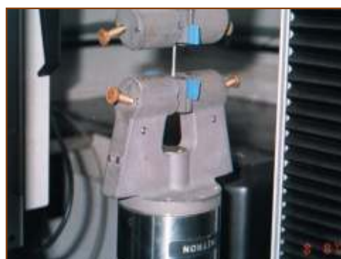
FIGURE 2 - Skin body test fixed in claws to test of tensile strength (Instron Machine)
