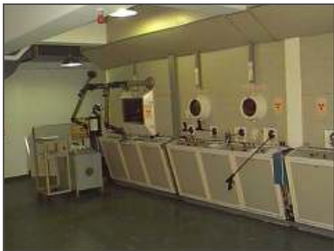
FIGURE 1 - Hot cells used for sealed source production.
