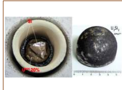
FIGURE 2 - Assembling of U_3Si_2 crucible load before melting and the resulting ingot after induction melting.
