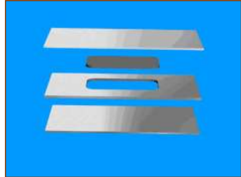
FIGURE 1 - Assembling set used to fabricate fuel plates involving the so-called picture-frame technique.
