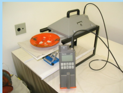
Figure 2. Apparatus for monitoring lightning rod plates
