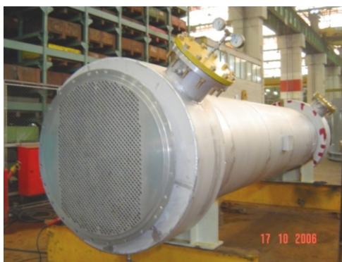
Figure 12. New heat exchanger
